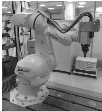
Figure 1. Industrial robot with 6 joints.
